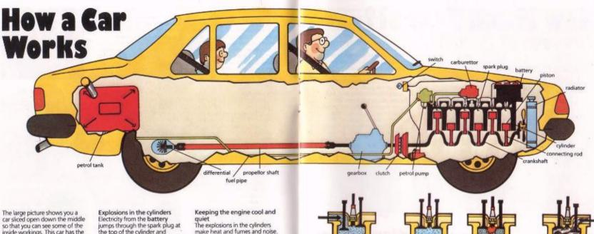
The large picture shows you a car sliced open down the middle so that you can see some of the inside workings. This car has the pengine at the front. In some cars the engine is at the back. The engine in this car pushes the back wheels round. How does the engine do the pushing?
